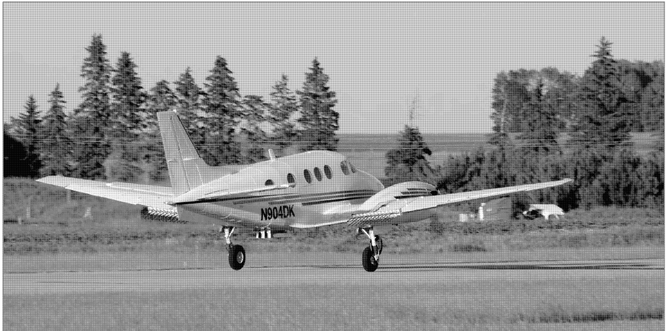
Fig. 21. A King Air model C90, Hailstop 1, takes off from the Olds-Didsbury Airport on the afternoon of June 6 th , 2017. Racks of burn-in-place pyrotechnics are visible aft of both wings. The three silver racks on the aft fuselage bottom each contain 102 20g ejectable flares. (WMI photograph by Adam Brainard.)
