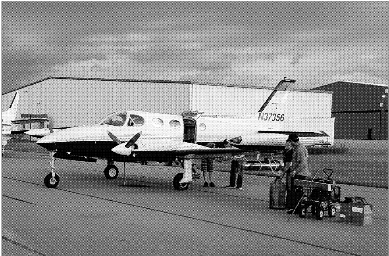
Fig. 22. A Cessna model 340A, Hailstop 4, rests on the ramp at the Red Deer Regional Airport, after the season's first days on which all five Hailstop aircraft seeded, June 9 th . The Hailstop 3 crew assists with reloading burn-in-place flares aft of the near wing, while the Hailstop 4 crew pumps additional seeding solution into the near ice nucleus generator. (WMI photograph by Mike Torris.)
