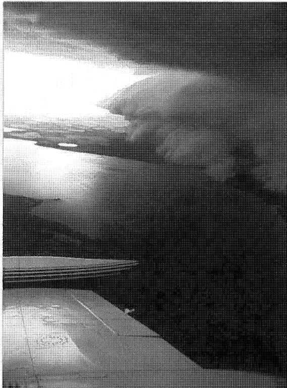
Fig. 7. Base seeding with wing-tip ice nucleus generators is conducted by Hailstop 2 in organized updraft beneath developing cumulus turrets on the flank of a mature thunderstorm. WMI photograph by Jacob Eeuwes.
