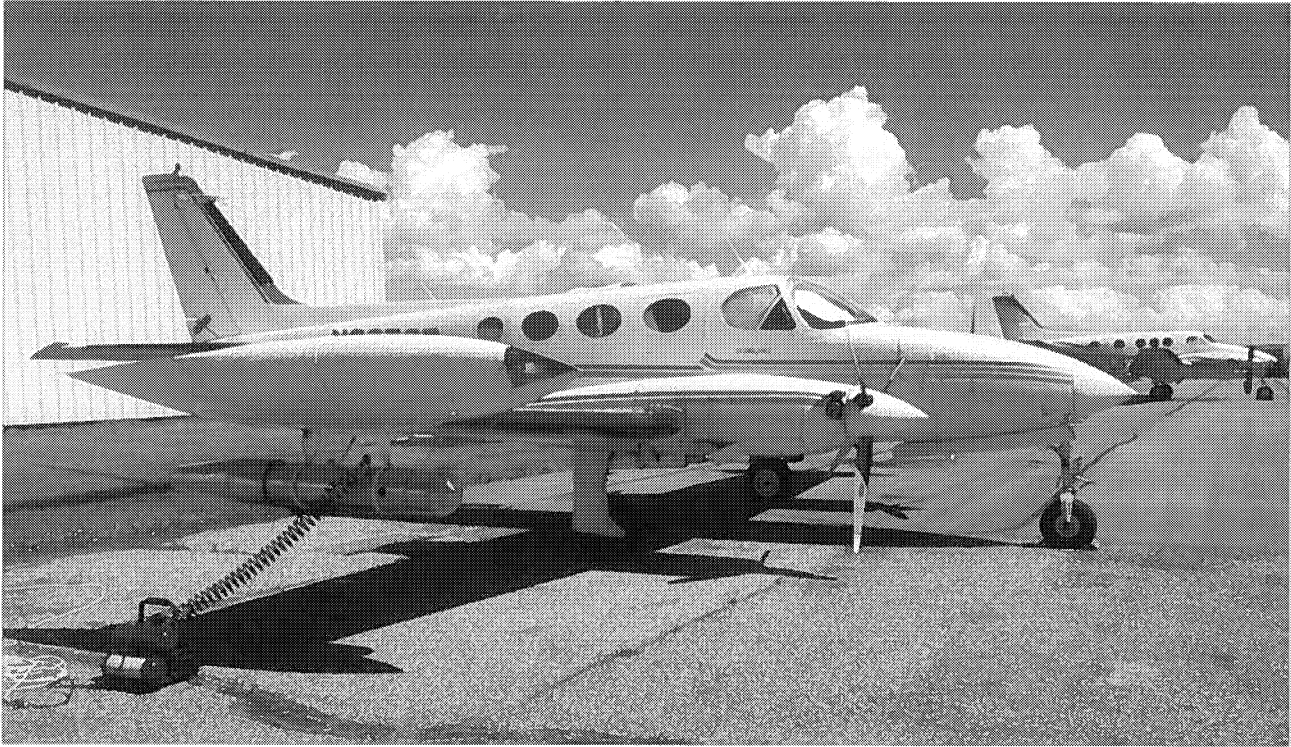
Fig. 19. Hailstop 4, a Cessna 340A seeding aircraft is shown on the ramp in Red Deer. Notable on the aircraft (and absent from the turboprop aircraft such as Hailstop 3, seen in the background) are the wing-tip ice nucleus generators, the silver torpedo-like appurtenances below the wing-tip fuel tanks. The photograph was taken just prior to the daily weather briefing, during preflight inspection. The compressor is used to fill a pressure vessel in the front of the generator that provides the flow of seeding solution to the rear, where it is burned. WMI photograph by L.J. Dunn.
