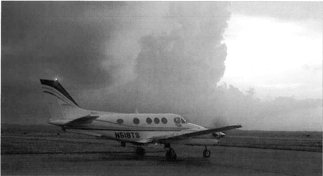
Fig. 18. Hailstop 1, one of three King Air C90 aircraft on project, taxis for takeoff at Springbank on August 12, 2013, at 8:12 PM. A "double-rack" of burn-in-place cloud seeding pyrotechnics is clearly visible aft of the engine on the near wing. The racks for smaller, ejectable flares mounted on the aircraft belly are more difficult to discern. WMI photograph by Brent Shewchuk.
