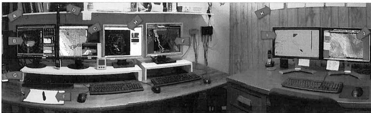
Fig. 20. The configuration of the Operations Room. Equipment includes (A) reference manuals, (B) TITAN displays, (C) CIDD, (D) VHF radio for communications with aircraft, (E) radar log, (F) internet data displays, (G) telephone, (H) AirLink display, (I and J) forecasting/nowcasting support displays, and (K) radio and radar licenses. WMI wide-angle photograph by Daniel Gilbert.
