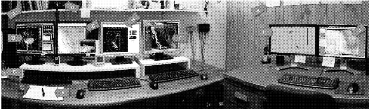
Figure 20. The configuration of the Operations Room. Equipment includes (A) reference manuals, (B) TITAN displays, (C) CIDD, (D) VHF radio for communications with aircraft, (E) radar log, (F) internet data displays, (G) telephone, (H) AirLink display, (I and J) forecasting/nowcasting support displays, and (K) radio and radar licenses. (WMI wide-angle photograph by Daniel Gilbert)
